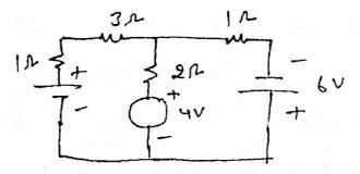
State Thevenin's Theorem. Determine the value of current flowing through 1 ohm resistance by using Thevenin's theorem.
